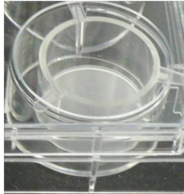
PET-Insert with defined pore size (1,0 µm)
