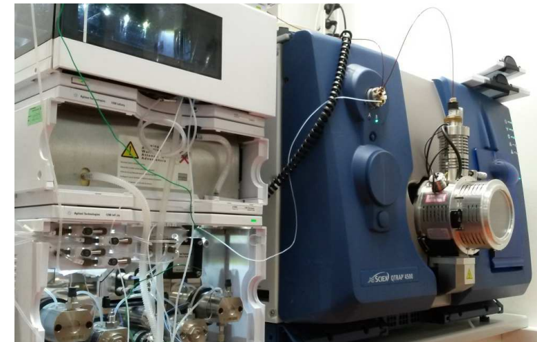
The LCMS/MS setup used to analyze the samples
